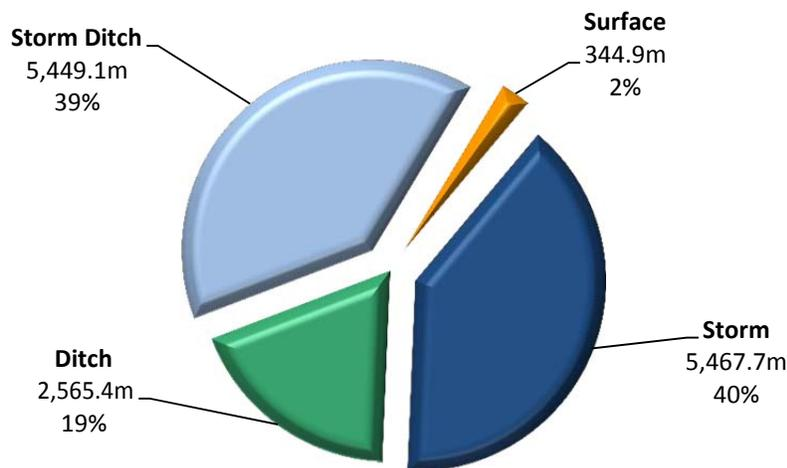
**Figure 2.2-1: Drainage System Types**
