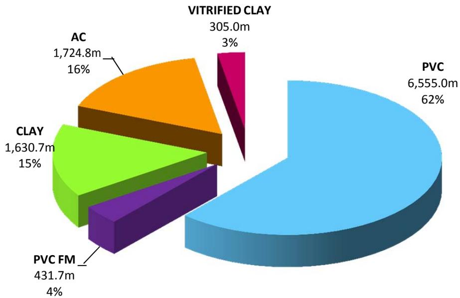
Figure 2.4-2: Sanitary Sewer Breakdown by Material
