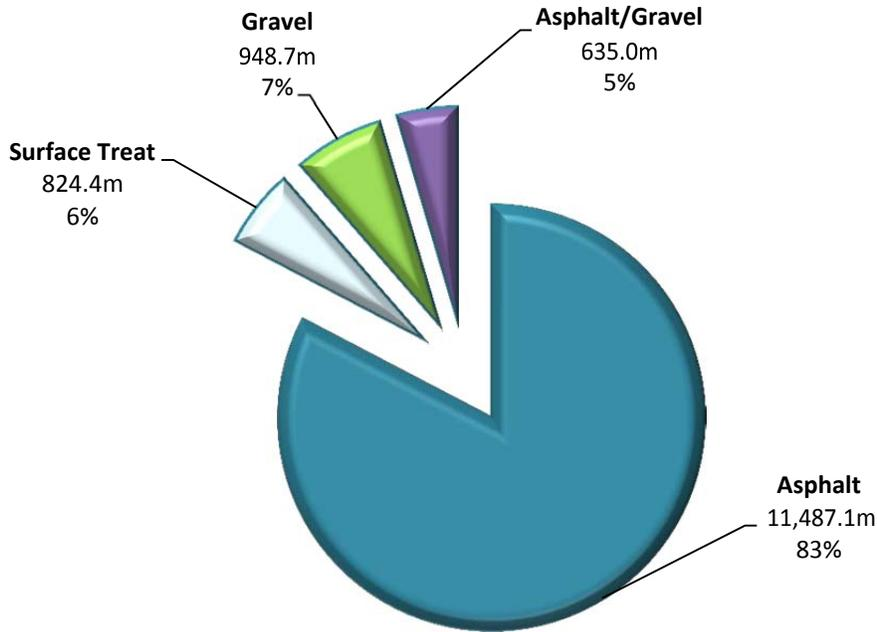
**Figure 2.1-2: Breakdown of Roads by Surface Type**
