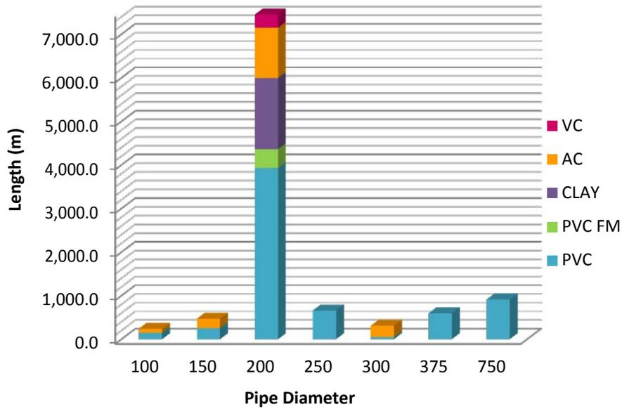
Figure 2.4-1: Sanitary Sewer Breakdown by Size and Material
